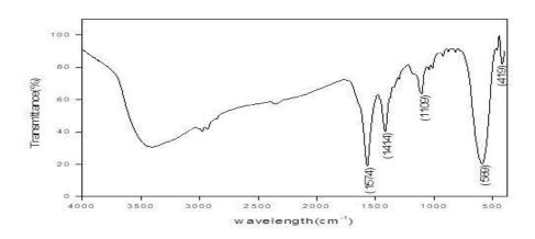
Fig. 2. FTIR pattern CuFe<sub>2</sub>O<sub>4</sub> nanoparticles
