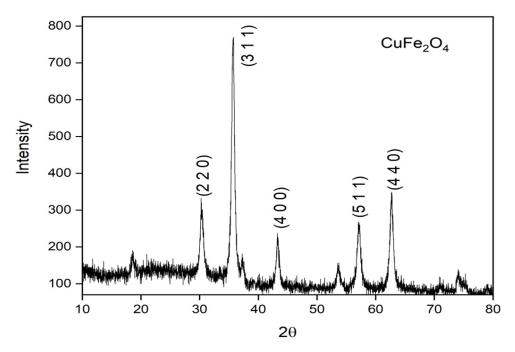
Fig. 1. XRD pattern CuFe<sub>2</sub>O<sub>4</sub> thin film
